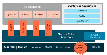
Cryptovision SCinterface consists of several modules. Some of them enable the addressing via crypto interfaces (MS-CAPI, CNG, PKCS#11, CryptoToken-Kit), others are used for administration.
